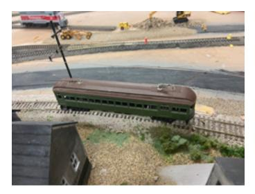
The overhead wire is .0125 bronze piano wire. The trolley is an old Bowser model that has been sitting on my shelf for fifteen years. It has the original Pitman motor that I rewired to run on the overhead.
